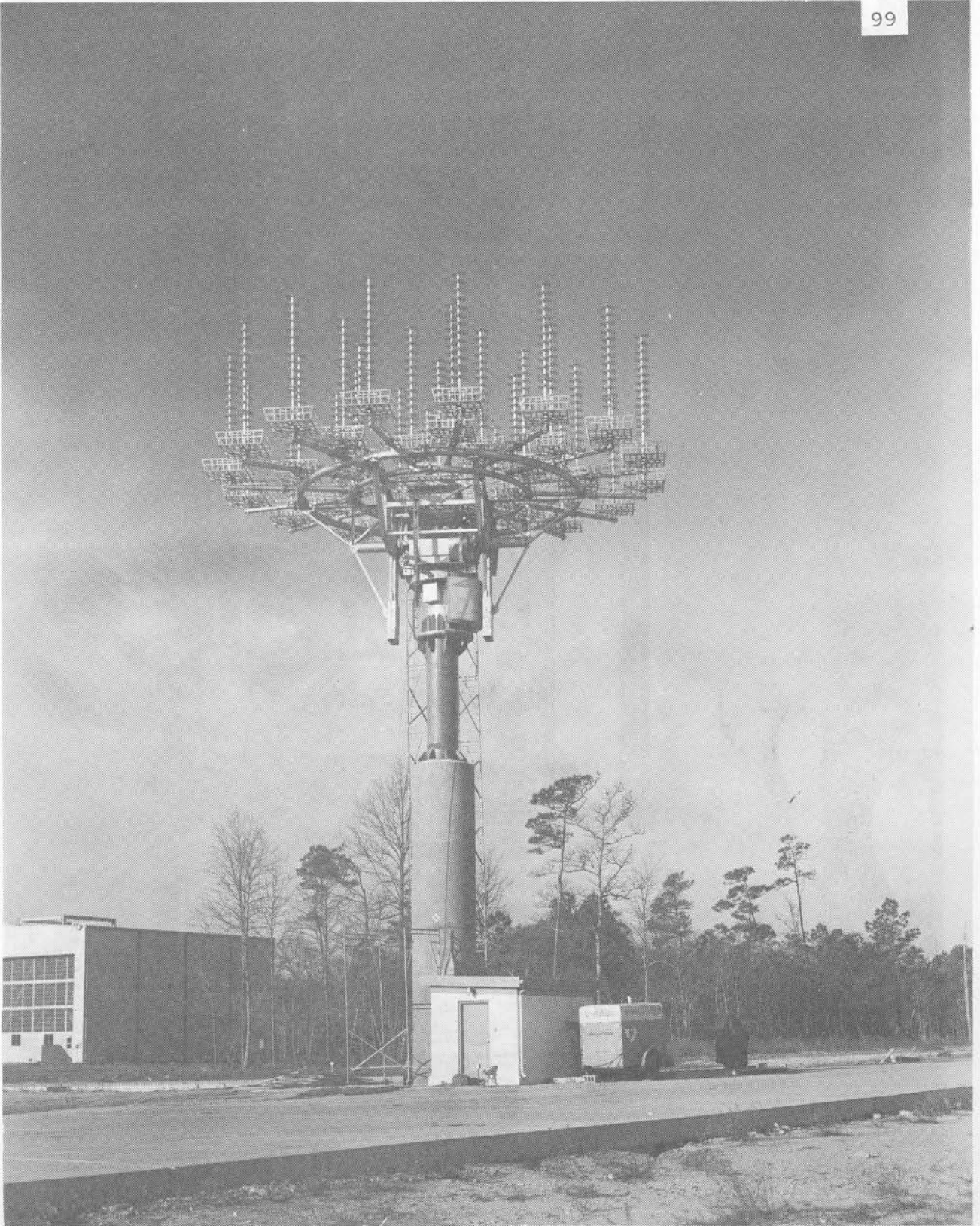
The high-gain, receiving antenna at NASA's Wallops Island facility used to receive data and track TIROS II. (NASA Photo)
