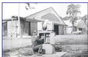
An unidentified airman inspects the ceilometer installed at Yokota Air Base, Japan, 1948.
