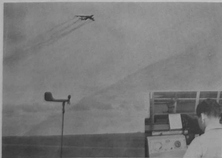
WIND-MEASURING SET at Manston AB, England, is the first USAFE installation of the AN/GMQ-11. The sensing element, left, looks like an airplane itself, the tail acting as a wind vane and the "prop" recording velocity. The miniature plane is connected by an underground cable to the indicator component, inset right, located in the control tower. The two dials indicate wind direction and speed respectively.
