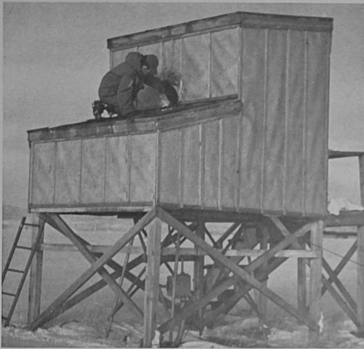
ONE OF THE TWO maintenance technicians of Detachment 5, TSgt John T. Phillips, checks the lens of the transmissometer projector to insure that it's clean and free from snow or ice. The transmissometer is located near the touchdown point on Runway 28 at Harmon AFB.
