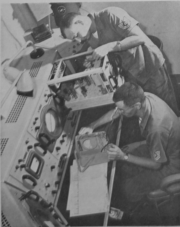
TSgt CLYDE L. HEYL, Maintenance NCOIC, and TSgt Royce N. Sanders trouble shoot a malfunction in the CPS-9 Radar Set.
