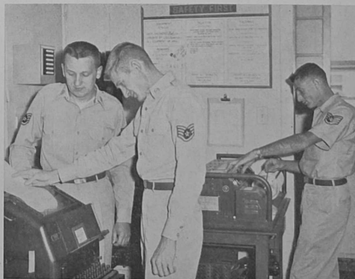
SSGT. MARVIN C. ALTMAN (center), ANG observer, checks the latest local teletype transmission under the watchful eye of SSGT Robert A. Janiszewski, AWS technical advisor to the 163d ANG Weather flight, while SSGT James E. Wolff, ANG observer, operates the facsimile machine.
