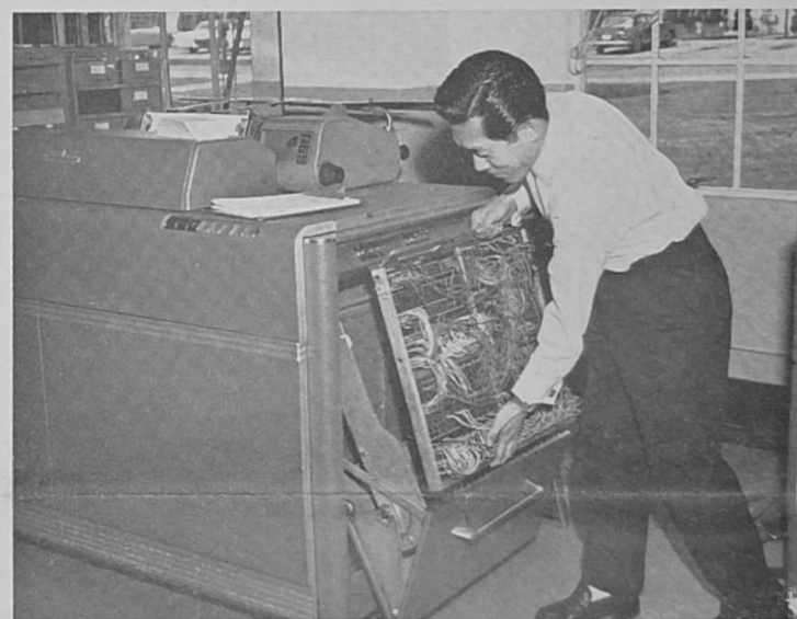
TAKING NO CHANCES that forecasters' predictions might decline in accuracy, Mr. George Taniguchi, weather consultant, inserts a control panel into an electronic tabulating machine, which in turn, will verify and score for accuracy, terminal forecasts that have been previously prepared.
