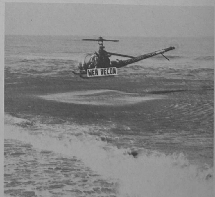
HOVERING over the Atlantic shore of Ft. Story, Va., is a OH-23 Raven helicopter. Chief Observer, TSgt Norman C. Craig estimates and records information on breaker heights and lengths of waves for radio relay.
