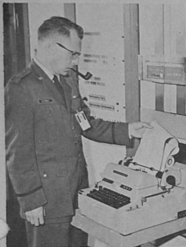
MONITORING readout from the Packard-Bell 250 computer in the meteorological office at Cape Canaveral is Capt. Evert A. Schmidt, Det 11, 4th Weather group. The computer processes micrometeorological data from the Cape-wide Weather Information Network Display (WIND) system.
