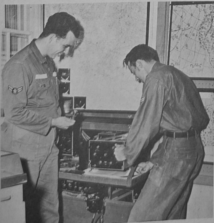
MAKING a preventive maintenance check of APQ-13 radar are A2c David W. Travis and A2c Robert D. Williams.
