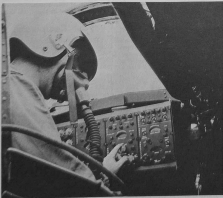
ADJUSTING weather equipment which will automatically take and transmit weather data to ground stations, is WB-47 co-pilot, Capt. Edward Giddings of the 54th WRS.
