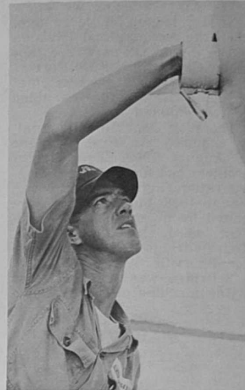
LOADING a dropsonde in the tail of a WB-47 is A1c William Anderson, a 54th WRS aircraft maintenance man. On a weather mission, the dropsonde is ejected from the aircraft by compressed air and automatically transmits weather data back to the aircraft.
