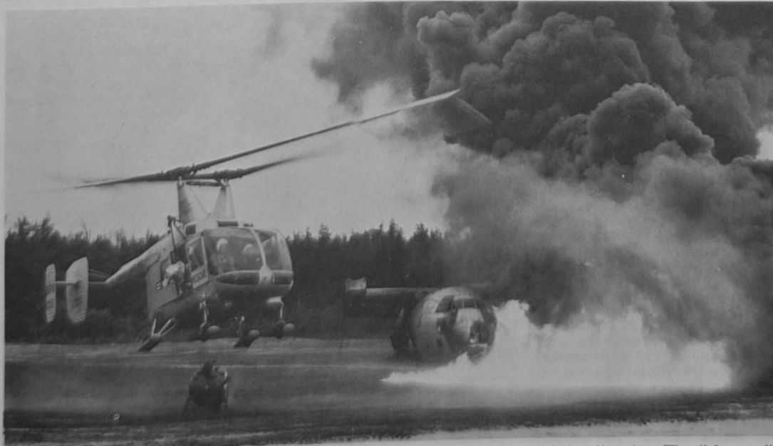
PRACTICING one of its most useful tricks is the HH-43B "Huskie" helicopter. The "chopper" can deliver the cylindrical fire suppression kit to the scene of an aircraft accident, transport firefighters, and hovering close to an aircraft fire, clear a path in the flames with its rotor wash so the firemen can get in close to work.
