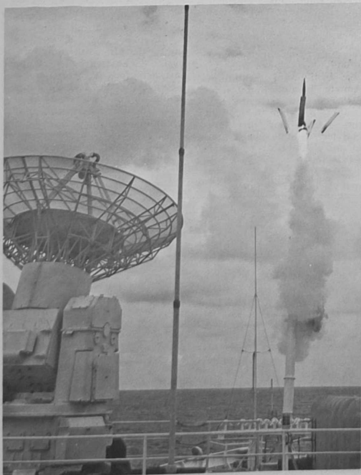
THAR SHE BLOWS...ER...GOES—The ARCAS meteorological rocket leaves the deck of the United States Naval Ship (USNS) Range Tracker on its 40-mile journey...straight up. Styrofoam spacers can be seen falling away from the rocket. (Air Force photo)
