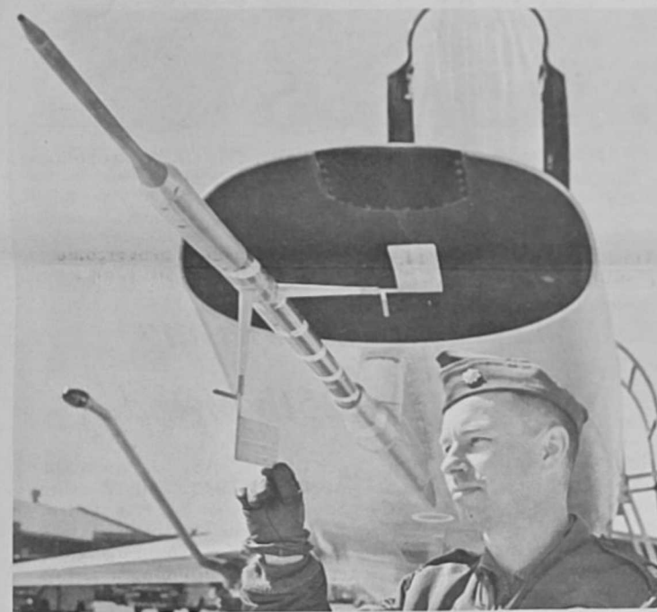
YAW VANE of the specially-instrumented F-100 aircraft is checked by CAT pilot, Maj. Robert J. Vanden-Heuvel, Aerospace Systems Division, AF Systems Command. The pitch vane can also be seen. Turbulence data obtained by these experiments will improve CAT forecasting techniques and minimize future aircraft damage or loss of life. (Photo by Maj. William H. Quelch Jr.)
