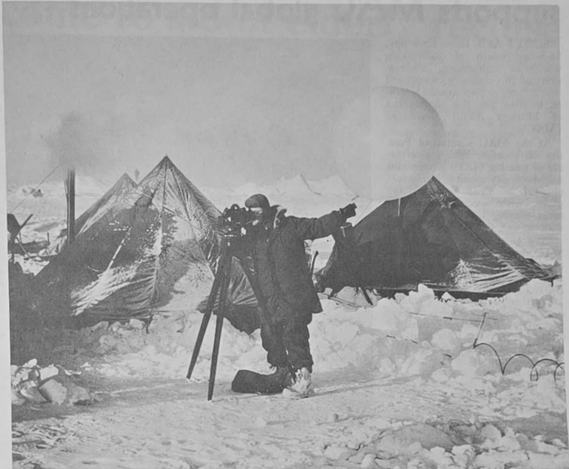
SIGHTING THE THEODOLITE prior to launching pilot balloon on the icy cape is SSgt. Michael A. Connell, NCOIC of the 172 Infantry Brigade Weather Team. Sergeant Connell was one of many weathermen who helped support the Alaskan Command exercise Ace Band Polar Cap. (U.S. Air Force Photo)
