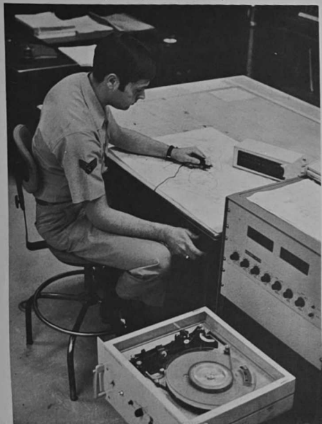
ELECTRONIC PENCIL follower, manipulated by Sgt. Gordon J. Brickner of AFGWC's analysis and forecasting section, transfers weather data from a manually drawn map to magnetic tape. When the resulting tape is fed into Global Weather's computer system, the computer can use the data to write and disseminate forecasts.
