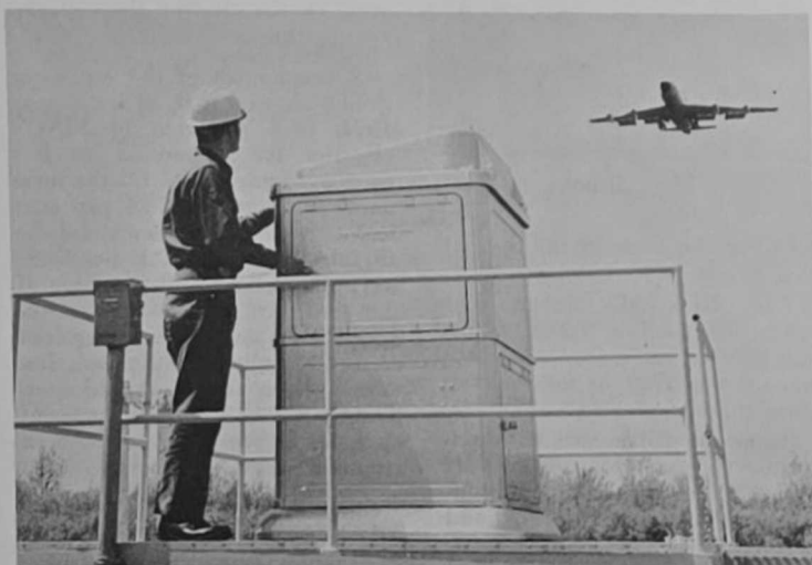
MAKING HIS DAILY inspection of the AN GMQ-13 rotating beam ceilometer is AWS maintenance man Sgt. Charles Henning of Detachment 2, 3rd Weather Wing while a C-135 aircraft lands at Offutt AFB, Neb. (U. S. Air Force Photo)
