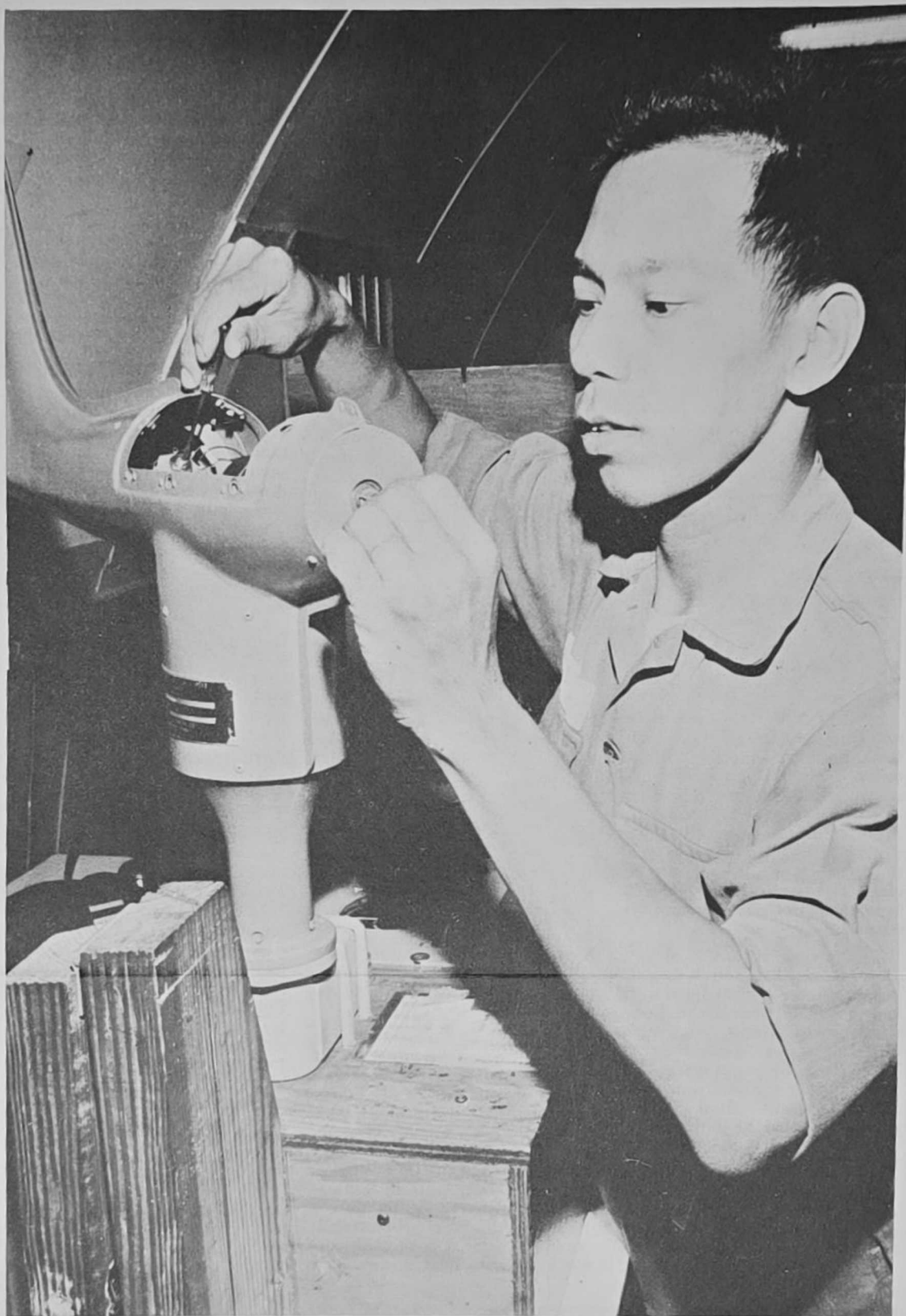
WIND SPEED and direction data is continuously provided by this wind-observing instrument being calibrated by VNAF TSgt. Nguyen Dinh Oanh.
