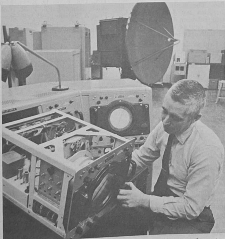
TROUBLESHOOTING the GMQ-10 transmissometer is part of the basic repairman's course. Participants, left to right, are A1c John H. Kune Jr., Instructor Roger A. Buchholz, A1c Ian A. Henry, Instructor Sgt. Craig D. Zimmerman and A1c Roy W. Funk Jr. and Michael J. Whitley.
