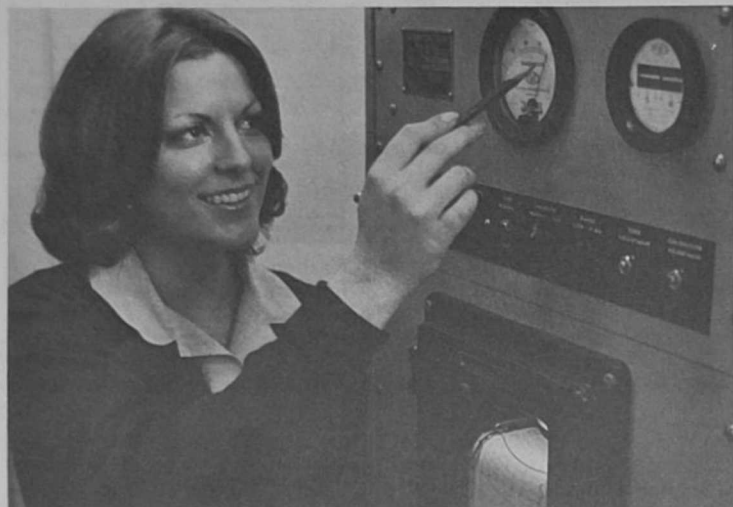
WORTH OBSERVING is Airman Janet S. Michael, student in the basic weather observer course. She takes a reading from the GMQ-10B transmissometer visibility-measuring set, during the 16-week course in which WAFs make up about 15 percent of the students.
