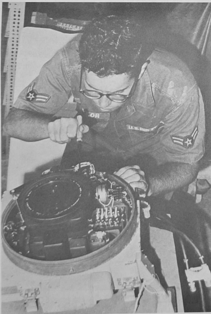
REPAIRING CAMERA, vital to squadron's mission, is A1c Michael A. Naylor, here making adjustments to an aerial mapping camera which takes 9x9-inch photos.
