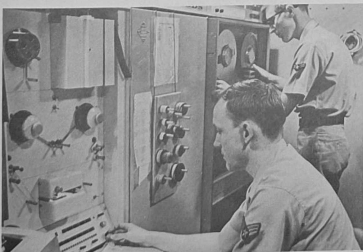
PROCESSING DATA, Sgt. Thomas E. Lamarre and Alc Patrick L. Holbert operate an SDS 910 computer, reducing data collected on an RC-130 photo mission.
