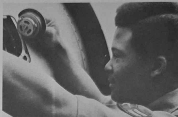
JET ENGINE mechanic McClain checks the oil on a WC-135 as part of the weather aircraft's post-flight inspection. The big AWS jet is the military version of the Boeing 707.
