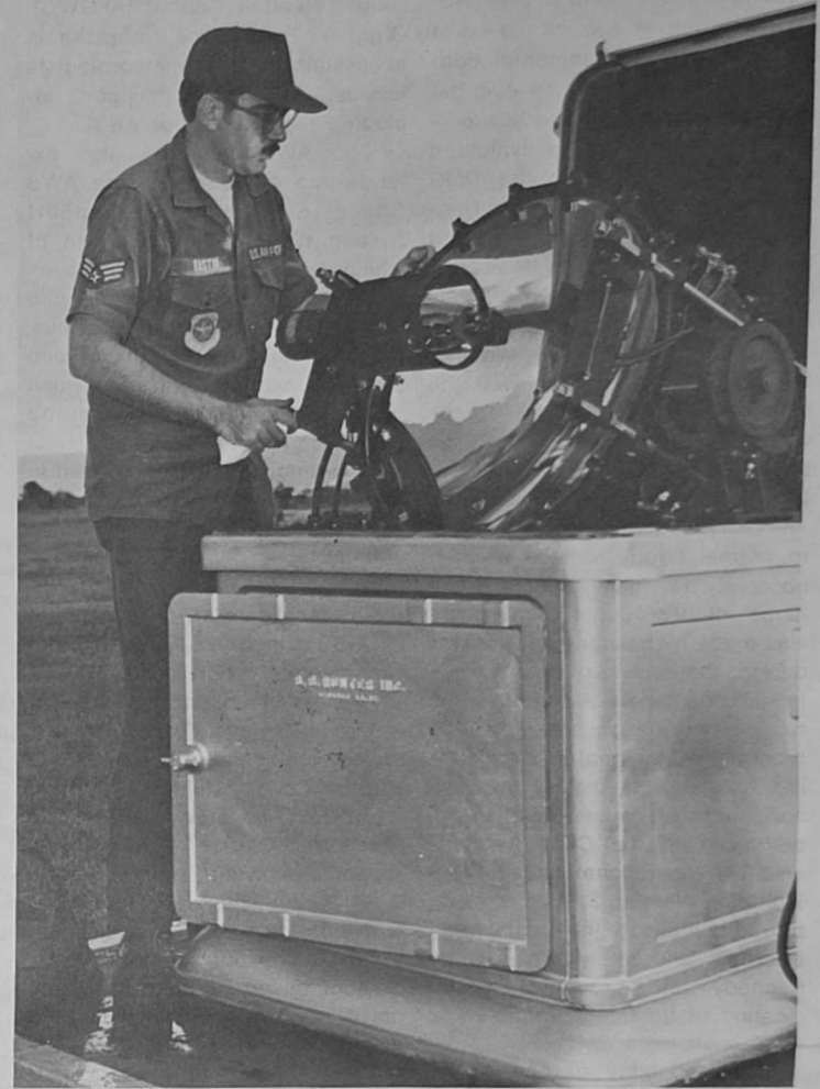
Sgt. Howard H. Eastin, who was recently named maintenance man of the year for the Air Weather Service checks instruments that are used to measure cloud height fall. Sergeant Eastin must make sure the device is operable 24-hours a day. (U.S. Air Force Photo)
