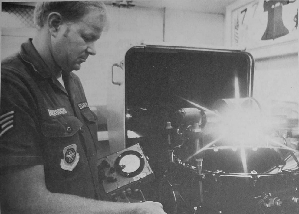
A FIVE MILLION candlepower beam is needed to allow the light to reflect off the base of clouds during measurement. The light is
