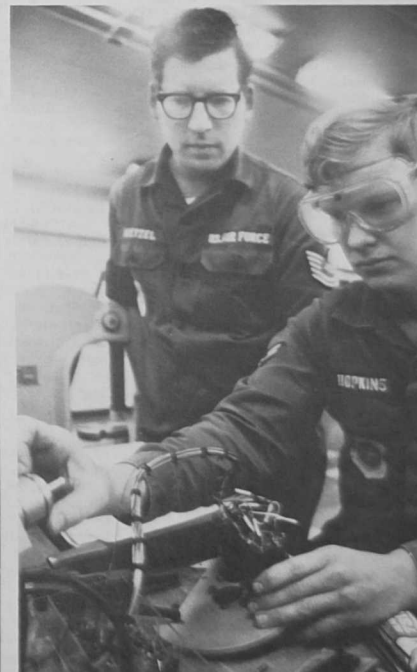
A1C LYLE HOPKINS reassembles an AN/FPS-77V weather radar pedestal with the guidance of his supervisor, TSgt. Julius Wetzel. Such operations are plentiful in Detachment 3, 1st Weather Wing, Yokota AB, Japan.
