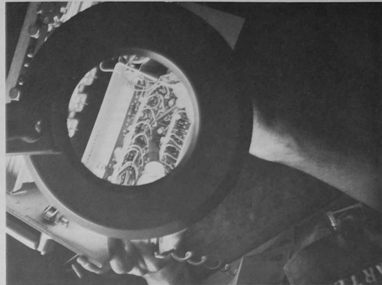
A BIRD'S EYE VIEW is given to solid state weather equipment being repaired by SSgt. Rick Hovarter. The view is through a circular magnifier, which is used for the "Little Big Jobs."
