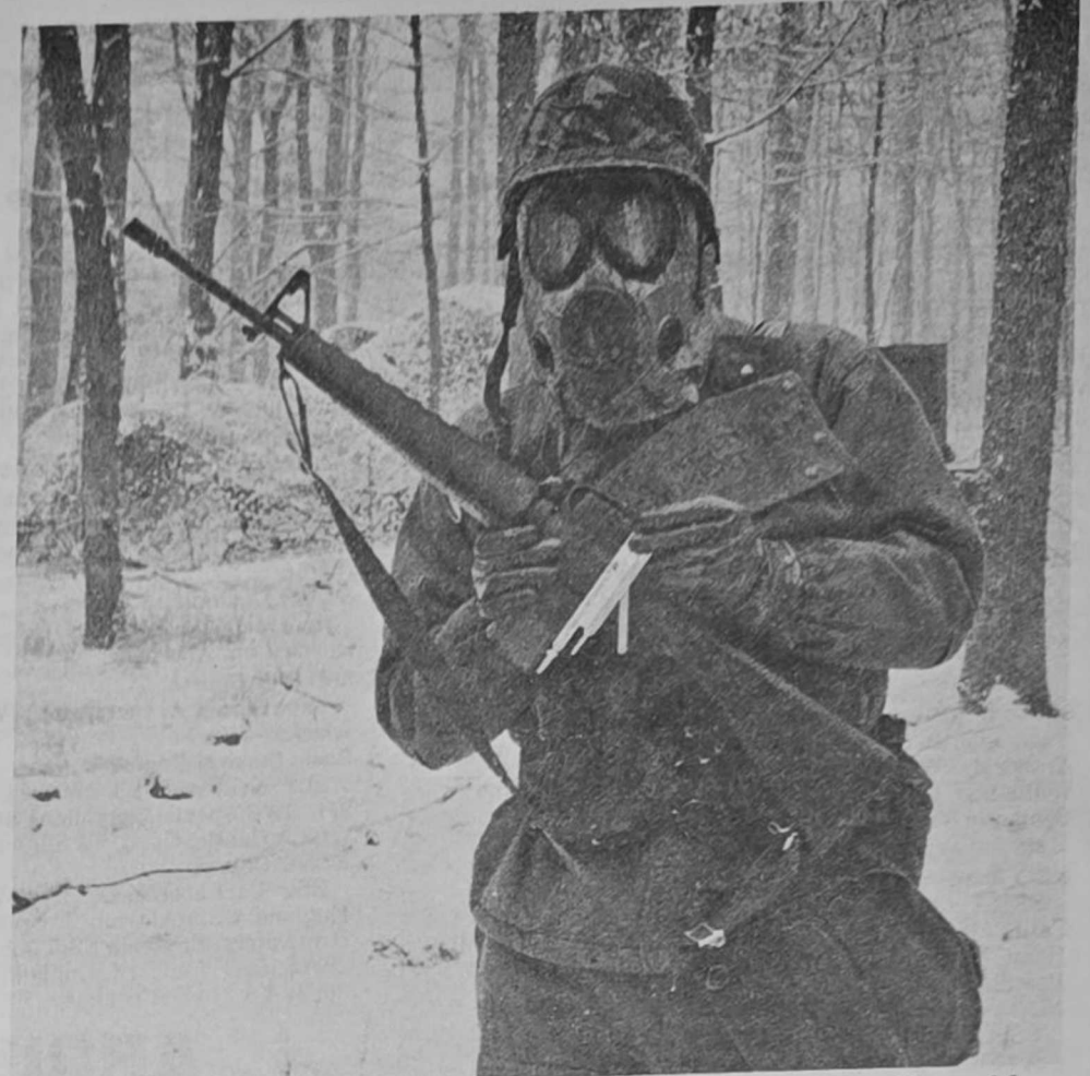
SSgt Robert W. Troastle taking a temperature/dew point reading with a sling psychrometer.
