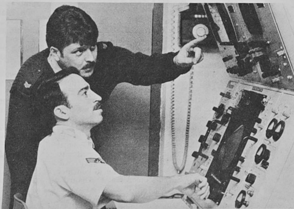
(Photo reprinted from the "Sentinel") SSgt. Brik Blackford discusses radar observation with Sgt. Eric Diaz at Det. 8, 31WS, Zweibrucken AB, Germany. Detachment 8's FPS-77 became fully operational last summer.
