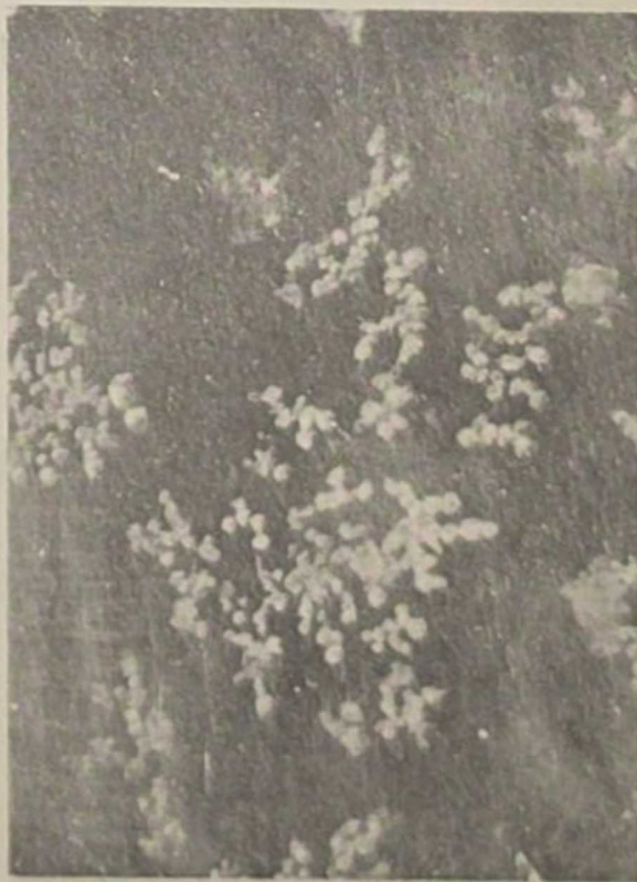
These small water droplets were photographed while rime icing was in progress. The liquid water content was only 0.2 grams per cubic meter, and the temperature, -20^{\circ}\text{C} .
