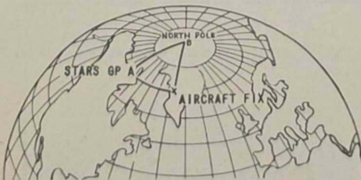
Figure 3: The Astronomical Triangle is used to compute the star altitude consistent with the Dead Reckoning Position, X; the side AX is equal to ( 90^\circ - \text{altitude} ). This side can be measured after reference to tables has permitted the plotting of side AB, angle ABX, and side BX.
